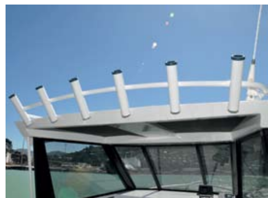
Left to right: The forecabin space is strictly stowage room; Designer Scott Robson (left) and Ramco owner Gary Tomes try out the movable bench seat: The six-position rocket launcher on the hardtop keeps the rods out of the way until needed.
