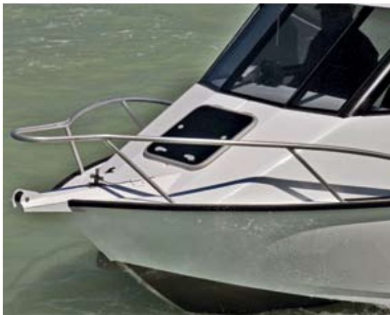
Left to right: the forward hatch offers best access to the bow for anchor duties; a wide entry allows easy access in
