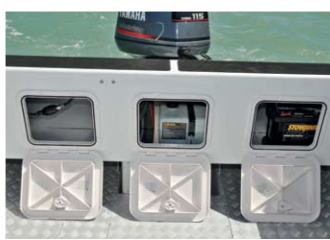
to the forecabin; as a dedicated day boat with no berths, the Ramco has heaps of cockpit space. Right: the battery and oil reservoir are protected up in the transom locker.
