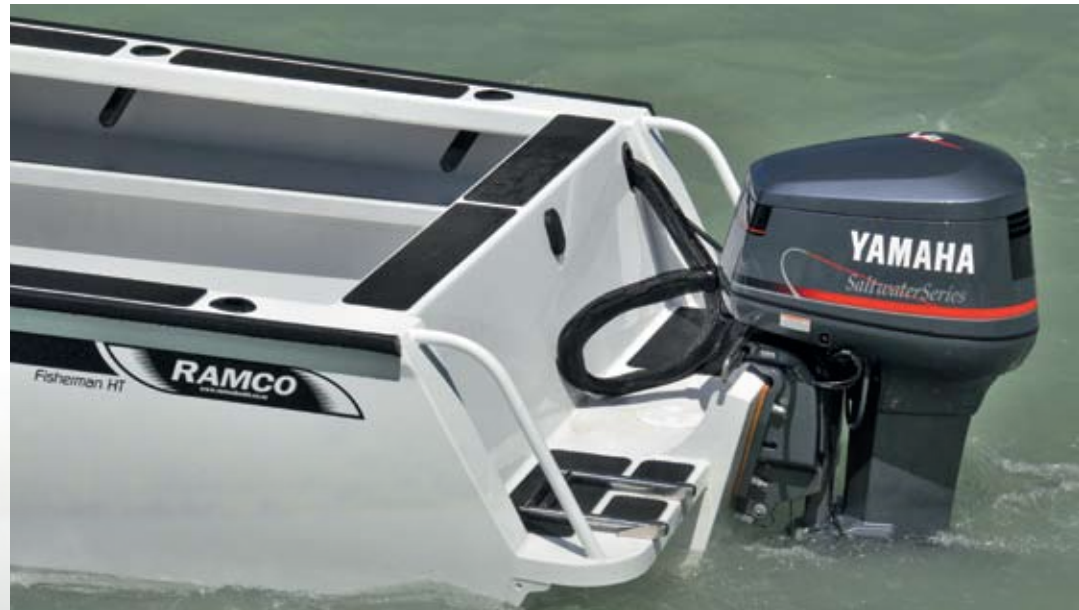
Left: clean lines and toe recess space makes the cockpit easy to fish from. Right: stern platforms feature grab rails and a fold-down ladder.
